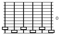
Below is the <u>worst</u> sort of curve to use because you are using EQ to *add volume*. With exaggerated boost you can easily run your power amplifiers into "clipping" (see page 5) and damage your speakers.
